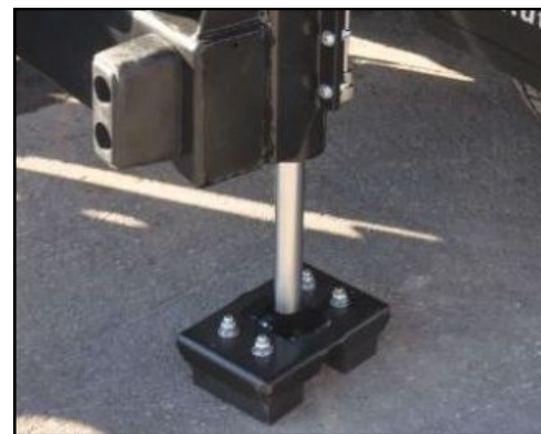
Stabilizers create a solid base for coring
