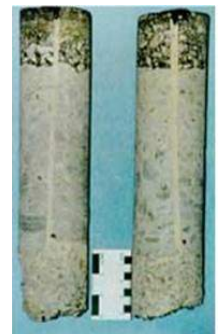
Figure 2. Satellite core samples taken through bonded area of rein-stated core. Light gray line, Utilibond™ shows excellent bonding of asphalt-concrete core (central area) and undisturbed pavement (outer layer) with complete infilling of voids in pea gravel (bottom). (See: Golder Report).
