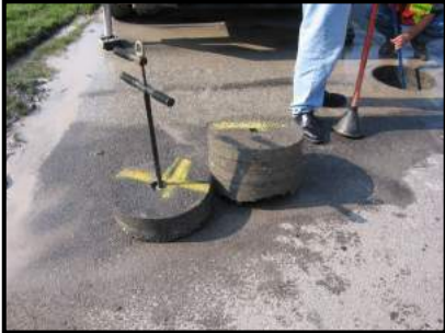
The Core shown above has been removed from the roadway. The layers of the core have separated. This is a delaminated core.
